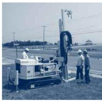
Geoprobe for soil and groundwater sampling
